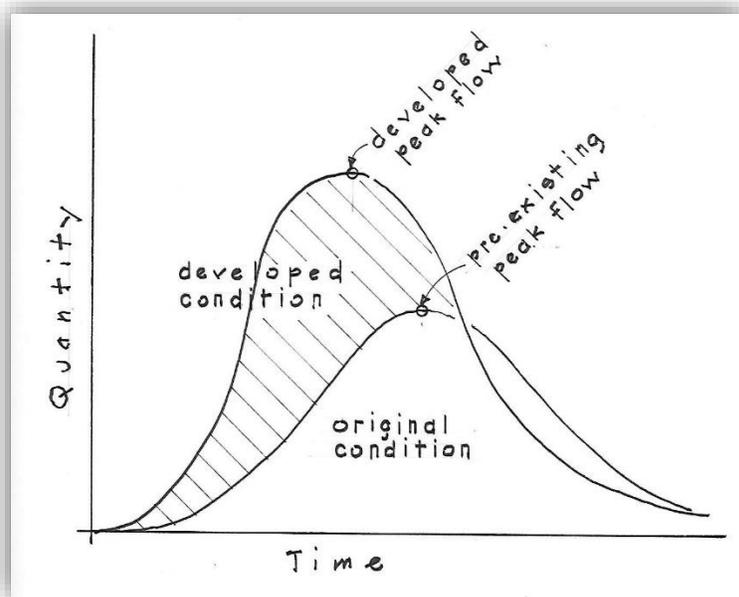
*Figure 1. The effect of hard paving on runoff. The intent of green design is to reduce the amount of runoff and lengthen its time back to that of its original state.*
