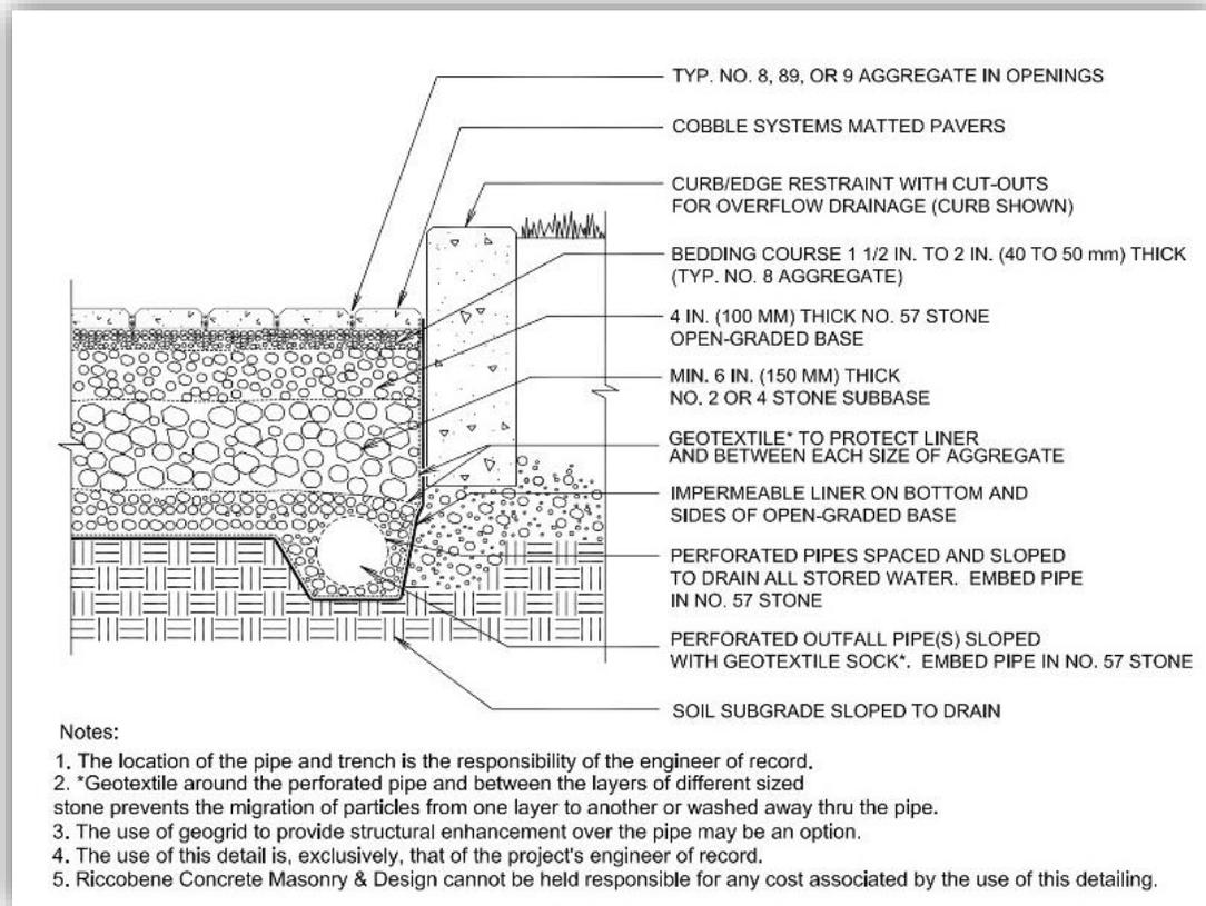
Figure 3. Typical permeable pavement with no exfiltration to soil subgrade.
